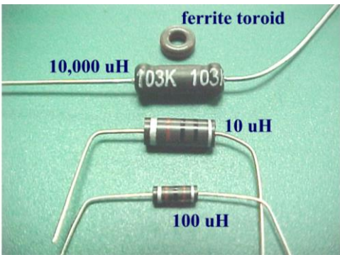
Figure A2 - Inductors and toroid.
